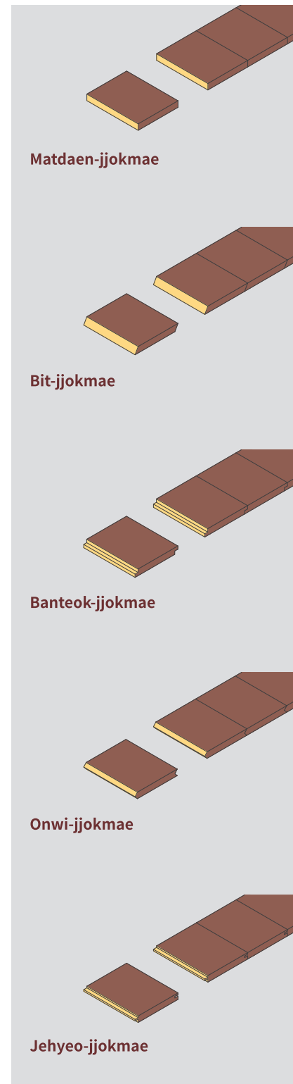
Types of floor joint
