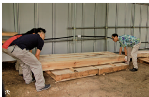
Storing timbers on a saw buck
