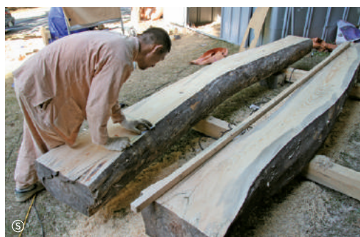
12 | Planing and cutting beam
